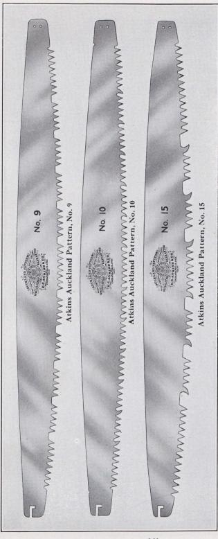
Nos. 9 and 48; space of teeth, all sizes, 1/4 inches. Space between sections of teeth, 2/8 inches. Space between sections of teeth, 1/4 inches. Nos. 10 and 49; space of teeth in 5-foot saws, 1 inch. All other sizes over 5 feet, 1/4 inches. Space between sections of teeth, 1/4 inches. Nos. 15 and 50; space of teeth, 6 to 7/2-foot saws, 1 inch; 8 to 10-foot saws, 1/4 inches. Space between sections of teeth, 2/4 inches.
