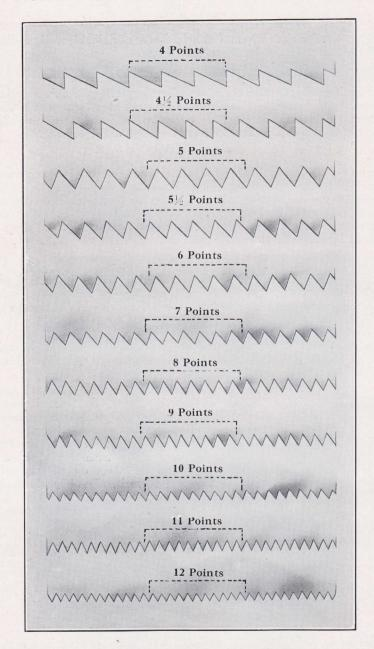
To prevent error in ordering, we are showing on this page a full-sized illustration of the various points of saw teeth from four to twelve.
