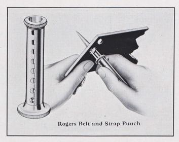
This punch is designed for cutting holes of any desired uniform size in leather or rubber belting, harness or similar material. The blade tapers and is curved. It slips into the handle when not in use and is withdrawn by pulling the thumb screw outward. A series of holes on the side of the handle regulates the amount of blade which is exposed and, therefore, the size of hole cut.
