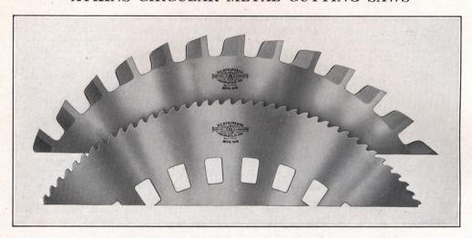
Blades for Bryant, and Q. & C. Machines have each tooth ground beveling on the rear, for clearance, and the blade is hollow ground. Gullets may be re-gummed when worn down. In ordering, give diameter, thickness, style of machine and class of material to cut. Spacing of teeth if possible, arbor and pin holes. For Higley Machines, state style of machine, class of material to be cut, diameter, thickness and pitch of teeth. Frequent sharpening is advisable in all metal saws to get the best results.
