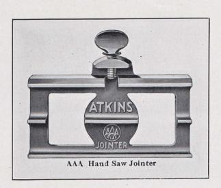
Atkins "AAA" Hand Saw Jointer is operated by placing a flat file in the Jointer, which is held in place by the thumb screw. The file is then passed lightly along the top of the Saw Teeth until it touches each tooth. The teeth are then filed to a point, thus securing teeth of the same length and shape.
