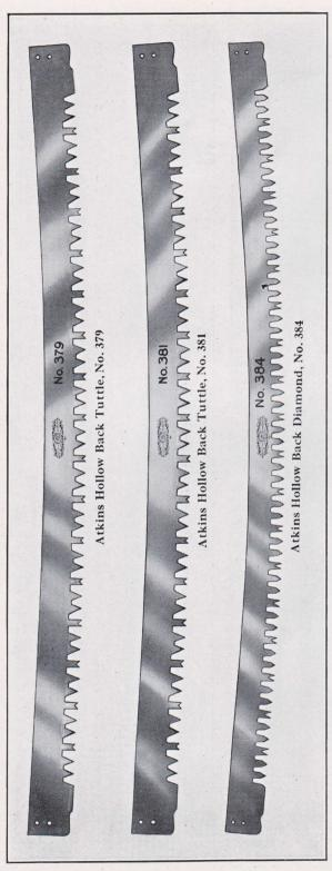
Atkins Hollow Back Tuttle, No. 379, is 3¼ inches wide at ends and center in all lengths. No. 380 is 3¾ inches wide, 13 or 14 gauge, No. 381 is 3¾ inches wide, 14 x 16 or 13 x 15. Depth of raker gullet, 1 inch. Width of raker gullet, widest place, ¼ inch. Depth of tooth gullet, ¼ inch. Width of tooth gullet, widest place, 15 inch.
