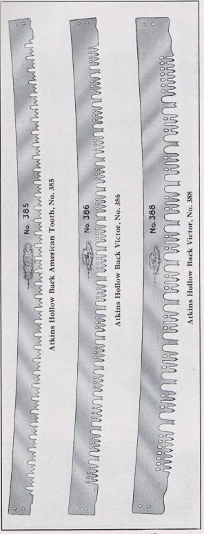
Atkins Hollow Back American, No. 385, is made in one width only, 3¼ inches at both ends and centers in all lengths. The depth of raker gullet is 1½ inches, width of raker gullet, widest place ½ inch, depth of tooth gullet ½ inch, width of tooth gullet, widest place ½ inch.
