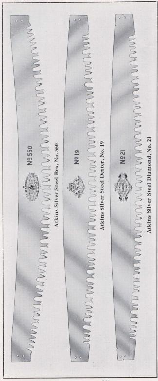
Segment ground. It is 14 gauge on toothed All saws on this page are made of Atkins Silver Steel. These features are fully described on pages 133 and 134. No. 550 has two cutting teeth, and a raker and is the "Finest on Earth" for cutting oak, and other hardwoods.
