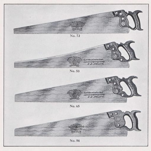
No. 72, Narrow Pattern. Silver Steel, Damaskeened, carved apple handle. The 26-inch blades are  $5\frac{3}{4}$  inches wide at the butt, and  $1\frac{3}{6}$  inches wide at the point. Other lengths are of proportionate widths. No. 53, Ship Carpenters. Silver Steel, skew back, Damaskeened, embossed and polished applewood handle, Perfection Pattern.
