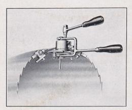
The Swage is made extra strong especially adapted for heavy work. The action of the Die is more of pressure than a roll. It duplicates the upper Swage for a strong corner, but it puts the spread of the steel on the under side. This Swage, used in connection with the Pribnow Shaper, has proved itself in putting up the strongest possible cutting point, besides effecting a saving in saw steel sufficient to pay for the outfit in a short time. This Swage is especially successful on Inserted Teeth.
